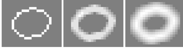
Figure 2: Example of “submanifold” dilation. Left: Original curve. Middle: Result of applying a regular 3 \times 3 convolution with weights 1/9 . Right: Result of applying the same convolution again. The example shows that regular convolutions substantially reduce the sparsity of the features with each convolutional layer.
