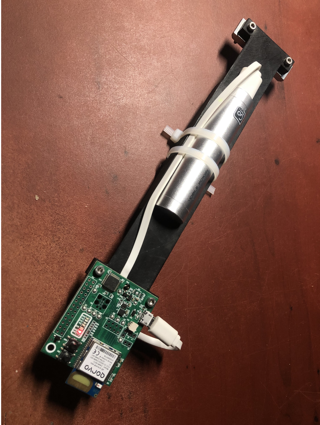
Figure 13: Final assembly for DWM prototype
